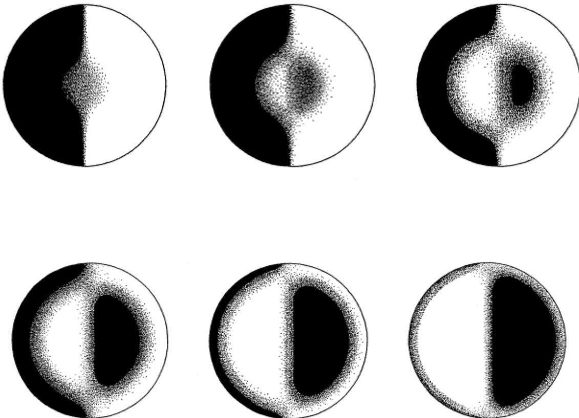
The total distance travelled by the knife edge from the image at top left to the image at bottom right is given by the formula:
