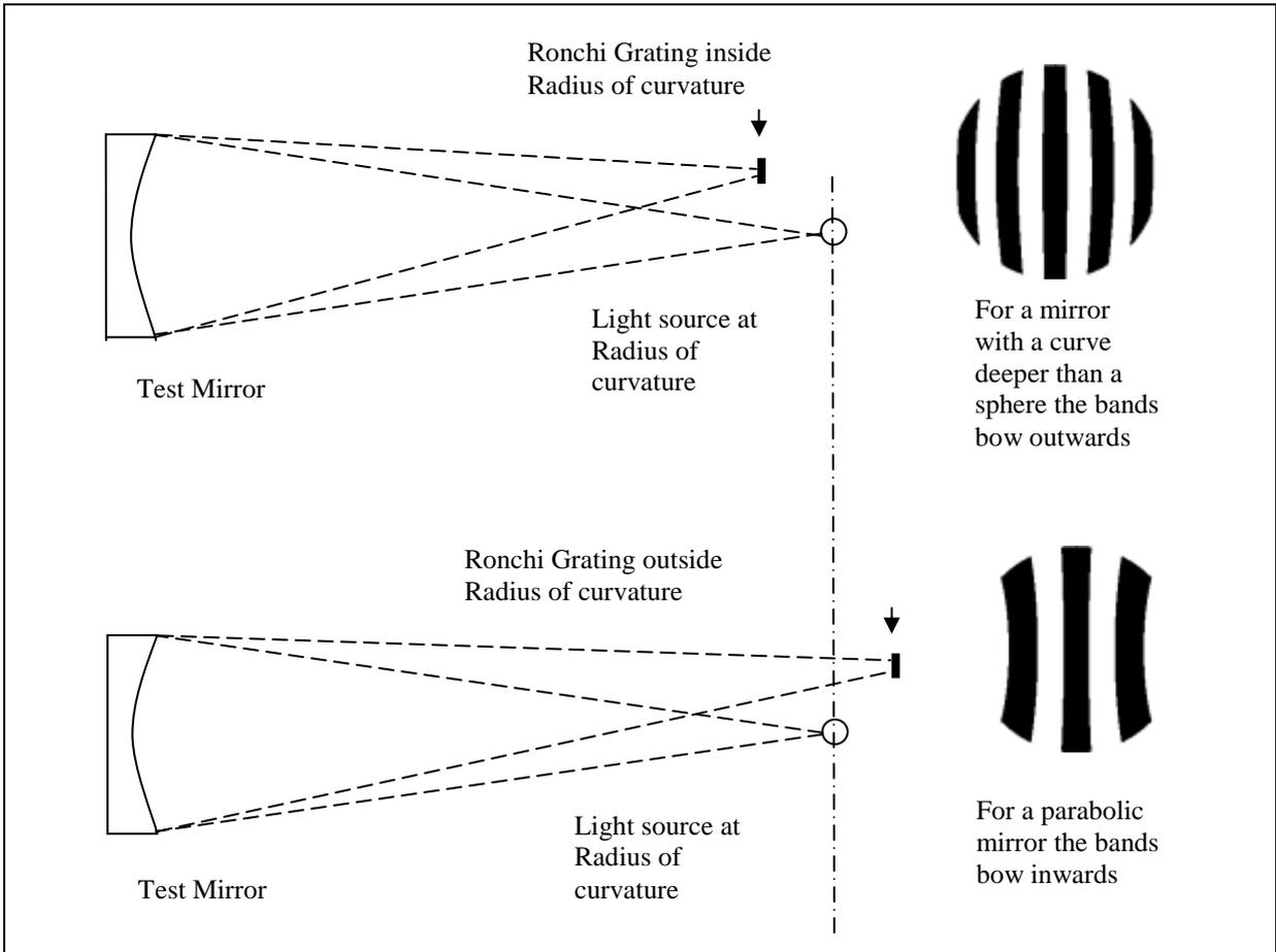
The ronchi band patterns can differ from being straight or curved depending upon the figure of the mirror being tested. The following table shows some real mirrors under the ronchi test together with an interpretation of what the images tell us about the mirrors
