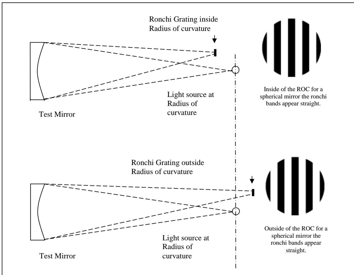
If the lines appear bowed outwards inside the ROC and bowed inwards outside of the ROC the mirror has a curve deeper than a sphere. It may be elliptical, parabolic or hyperbolic. As stated the Ronchi test is not quantitative, observing the curved bands does not enable us to say which conic section fits the mirror's surface.
